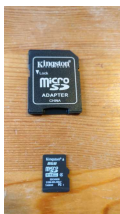
Micro SD card with a SD card adapter. Click for a bigger version. Picture taken by HagssFIN.
