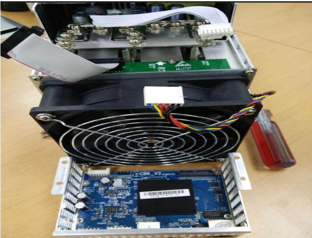
4) Remove the four screws fixed on the bracket and take out the control panel from the bracket as shown:
