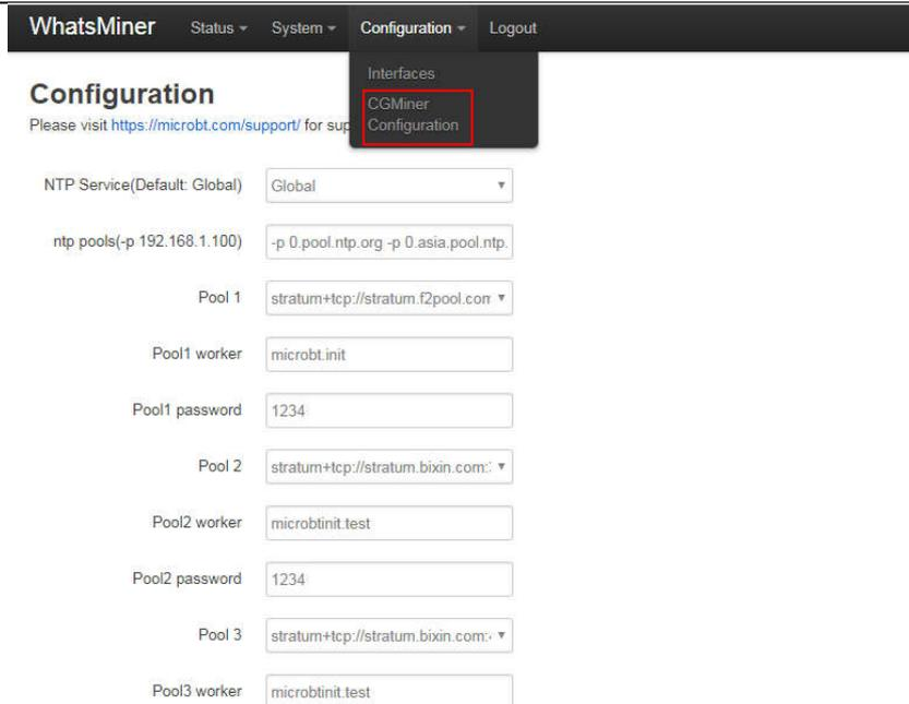
(2) In the cgminer configuration interface, add or modify the NTP server address. The miner has been configured with four NTP server addresses by default. You can modify or add the NTP server address to the local NTP server address according to the mine situation.
