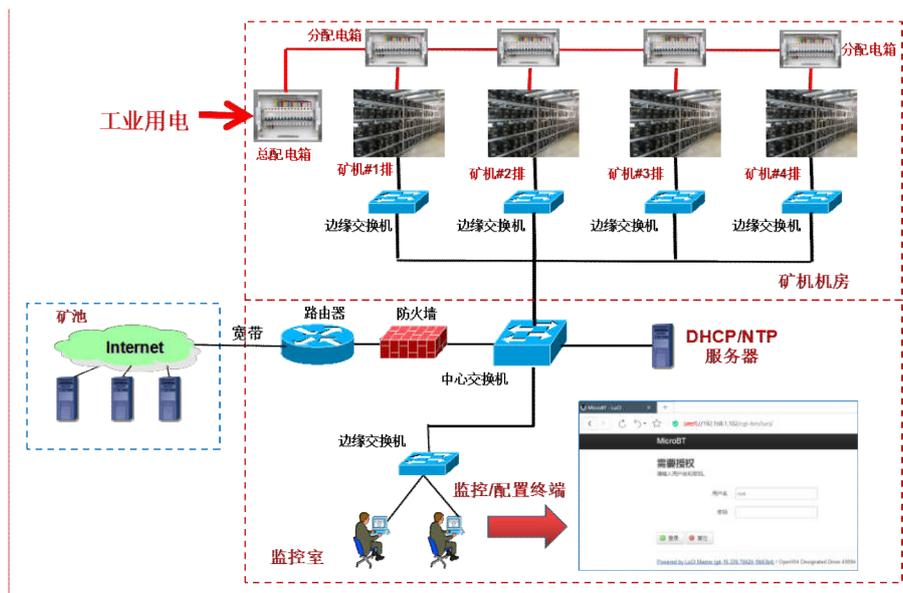
The miner defaults to DHCP to obtain dynamic ip. Therefore, the mine network must be configured with a DHCP server, or the router can enable dhcp to dynamically allocate the IP address service. The running time of the miner, the
