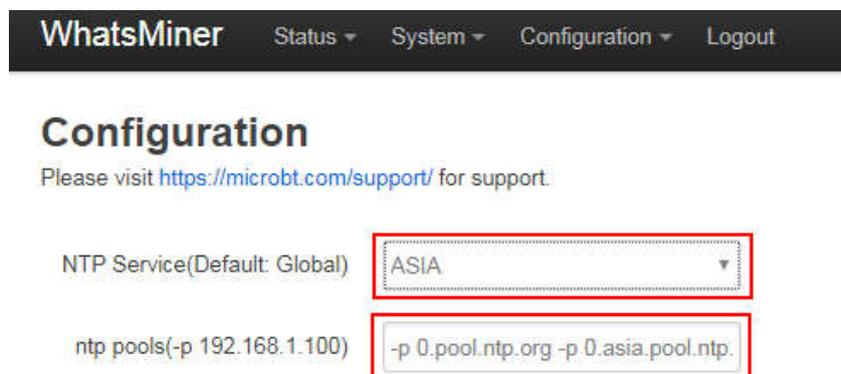
Default NTP server configuration: -p 3.asia.pool.ntp.org -p 2.cn.pool.ntp.org -p 1.cn.pool.ntp.org -p0.cn.pool.ntp.org
