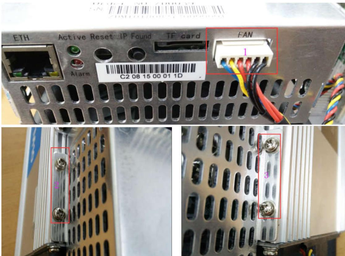
2) Unplug the fan and remove the screws as shown:
