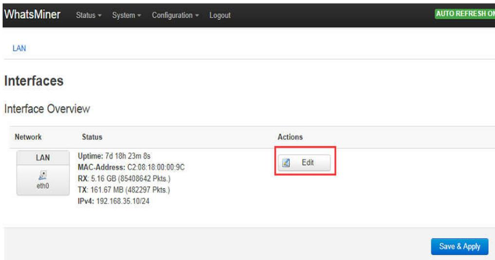
The screenshot shows the WhatsMiner web interface with the 'Configuration' menu selected. The 'Interfaces' section is visible, and the 'Edit' button in the 'Actions' column of the 'LAN' network row is highlighted with a red box. The 'Interface Overview' table shows the same details as the previous screenshot. A 'Save & Apply' button is at the bottom right.
