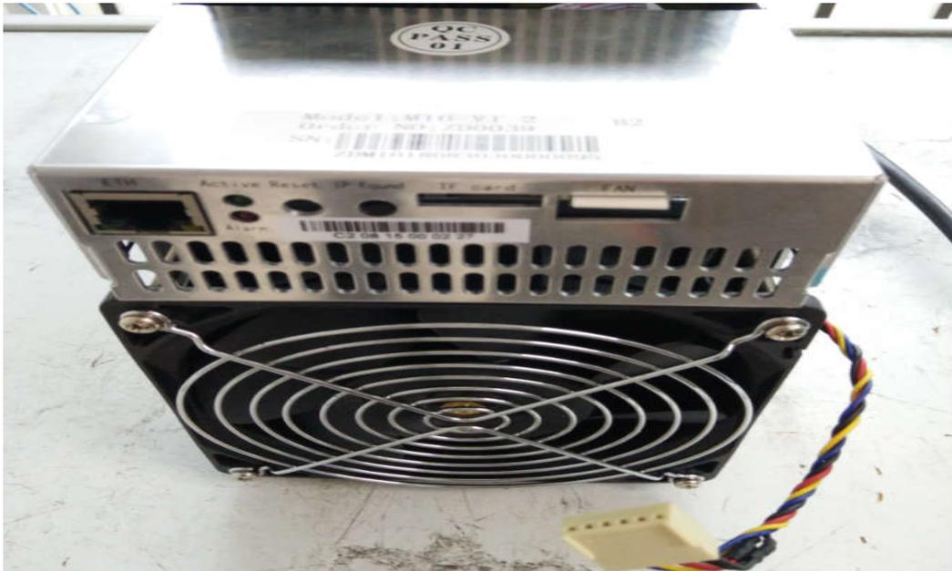
3) Plug the fan cable and the control board is installed.
