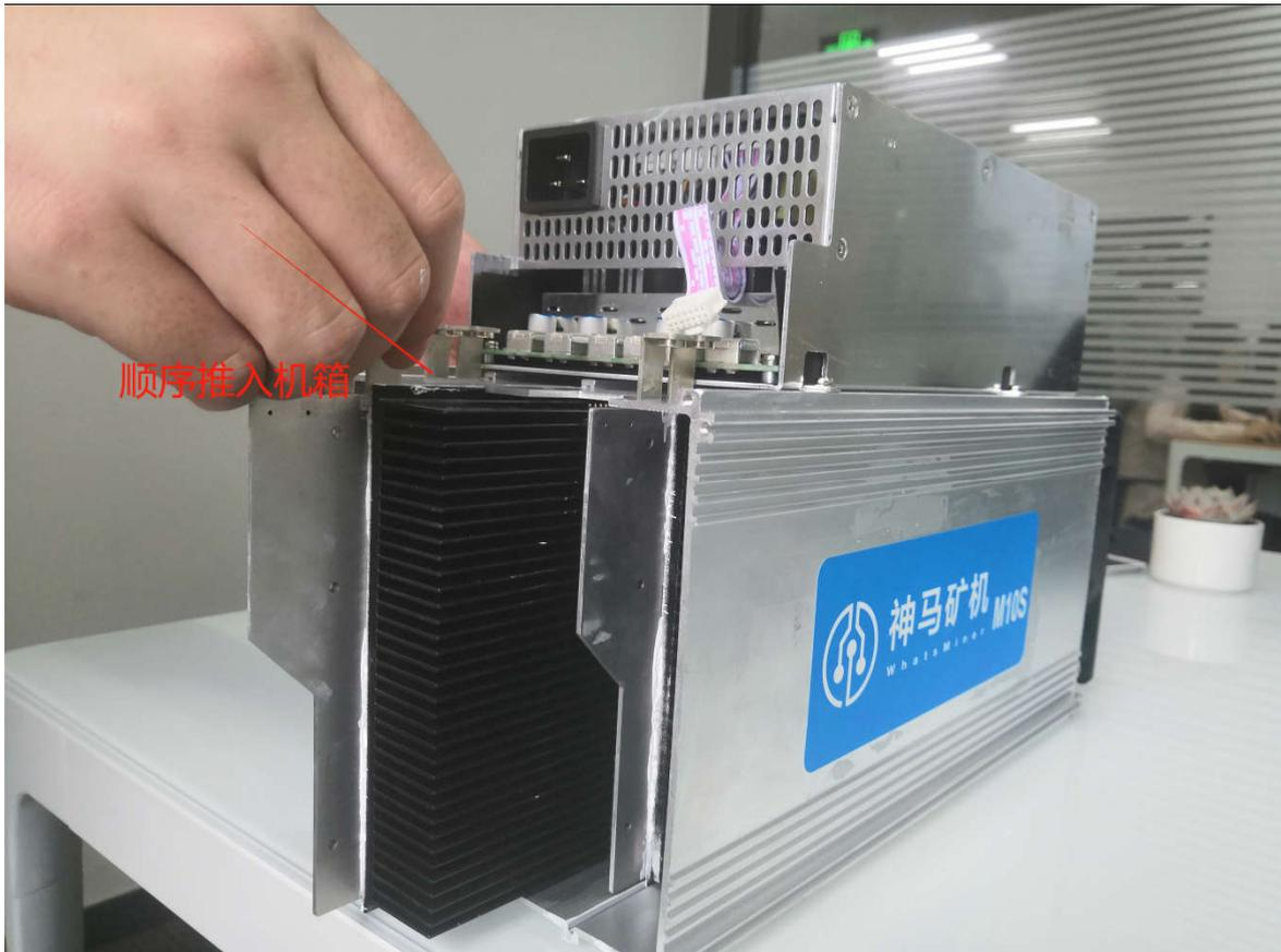
2) After installing the hash board into the chassis, first install the adapter board. The socket of the adapter board and the pin of the hash board must be installed in place to avoid other problems caused by contact problems, as shown:
