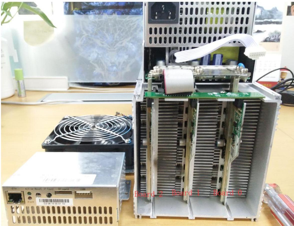
2) Remove the adapter plate and the copper bar fixed to the control panel as shown:
