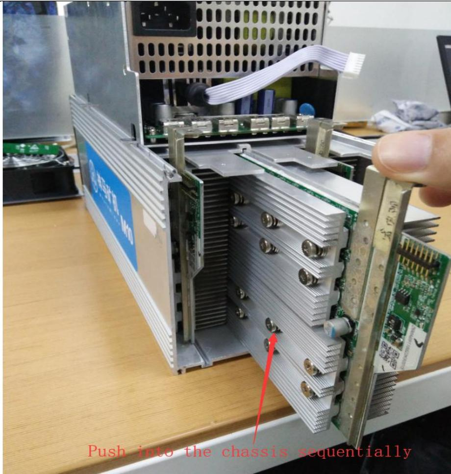
2) After installing the hash board into the chassis, first install the adapter board. The socket of the adapter board and the pin of the hash board must be installed in place to avoid other problems caused by contact problems, as shown:
