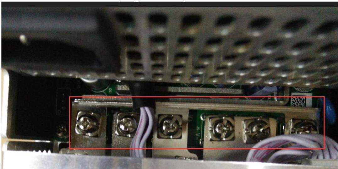
3) Finally, tighten the screws of the four fixed power supplies on the chassis, and the power supply is installed, as shown below:
