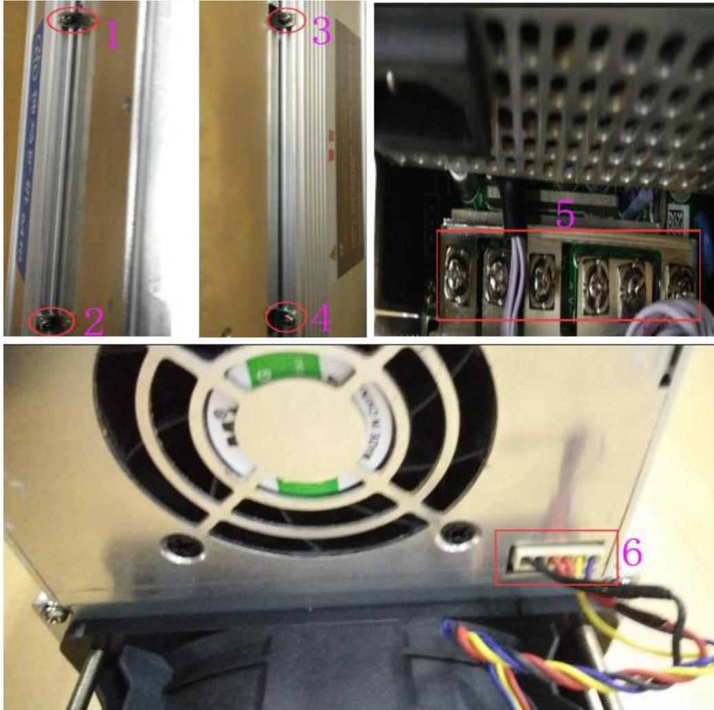
2) After the above operation is completed, gently pull out the power supply (do not pull out too long, the power control cable is still connected to the control panel), as shown in the figure:
