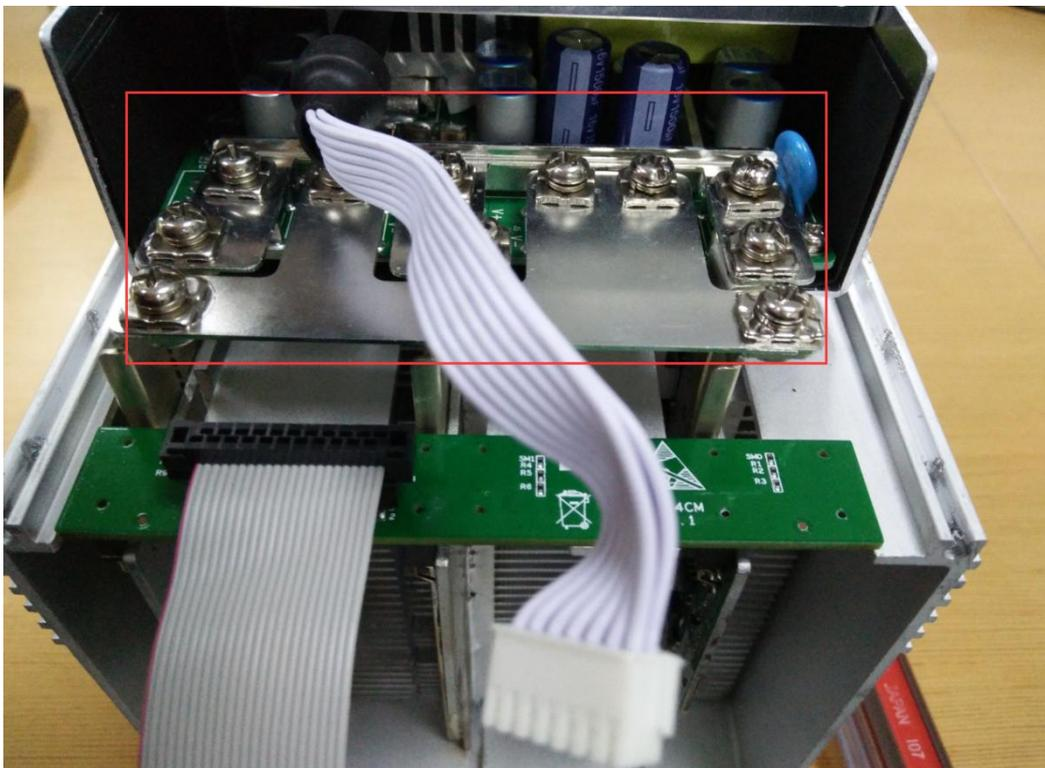
4) After the copper row is installed, the control board and the fan are installed, and the hash board is installed, as shown:
