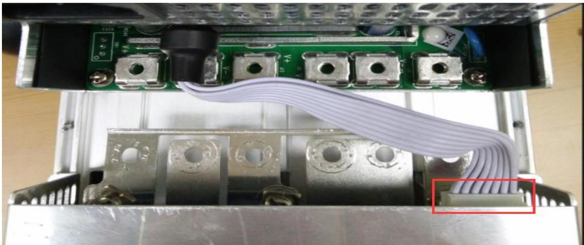
2) Then connect the 6 positive and negative terminals on the power supply to the copper row one by one, and then install 6 screws in turn. The screws should be tightened and the washers should be aligned parallel to the edge of the copper bar to avoid short circuiting the power supply or the power board, as shown below:
