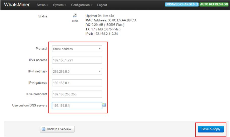
**After saving the application, you need to re-use the newly set static IP address to log in to the mining machine (otherwise the page will display as loading until the loading fails).**
