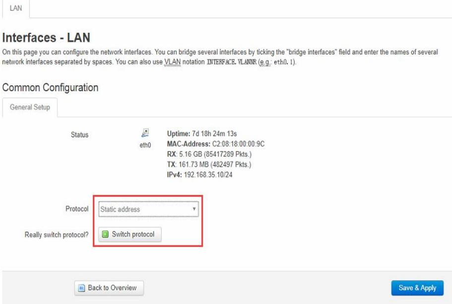
(5) In the static address configuration interface, change the IP address, mask, gateway, broadcast address, and DNS address to the actual planned address of the mine. After editing, click "Save & Apply" in the lower right corner.
