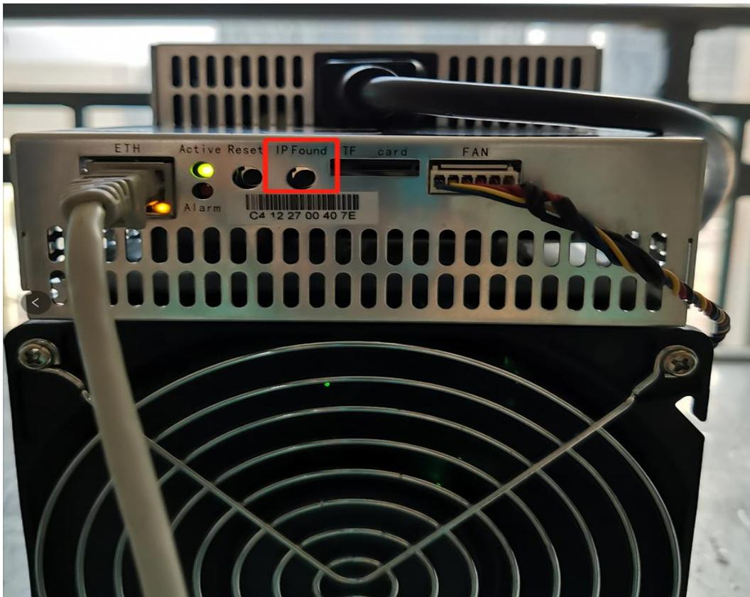
(2) View the dynamically obtained IP, MAC address, and miner position reported by the machine in WhatsMinerTools software.
